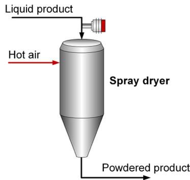
The K-Patents refractometer is used for monitoring the concentration of the feed line to the spray dryer. This measurement point is necessary to ensure the correct particle size after drying, and to increase the final product shelf life. An efficient drying operation also improves packaging by having the correct bag size and less weight due to the moisture.
