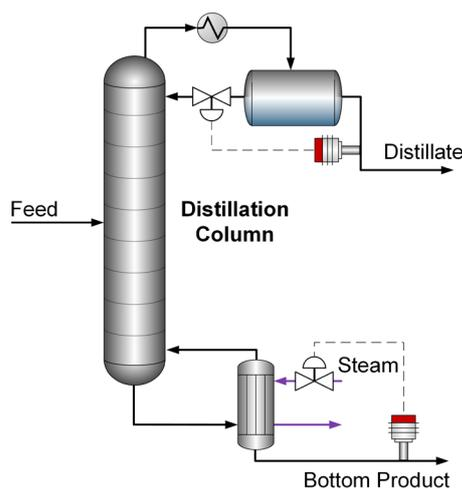
Distillation is one of the most common and important unit operations. In distillation, a mixture of chemicals is separated into its pure components based on their unique boiling points. Control of distillation is essential to meet product specifications, reduce investment and energy costs and limit environmental impact. These goals can be achieved by maintaining the purity of the column's top and bottom products within
